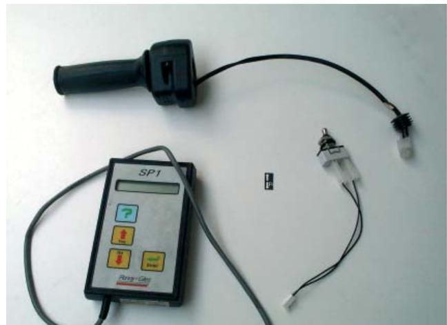
Figure 2: Twist grip throttle, left, and programming unit.
