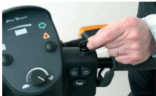
Figure 4: Remove the rubber plug.
