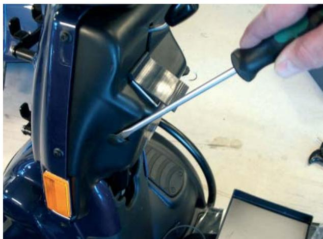
Figure 2: Remove the rubber plug from the plastic cover.
