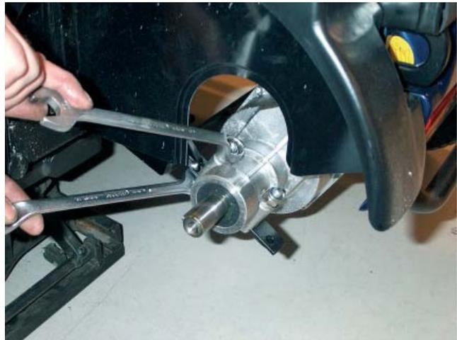
Figure 4: Loosen the rear M10 bolt. Remove the front bolt.
