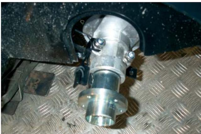
Figure 5: Use a self-locking nut when installing the holder for the magnetic sensor.
