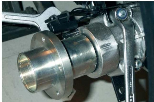
Figure 6: Install the sensor with a rubber gasket around the holder.
