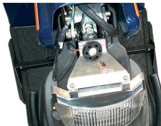
Make sure that the wires are not pinched when replacing the front shroud.
