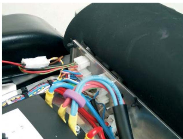
Figure 4: Attach the other plug from the hour counter to the PCB.
