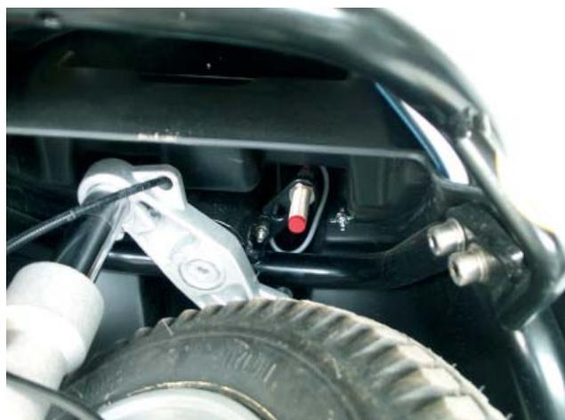
Figure 4: Install the sensor in the holder.
