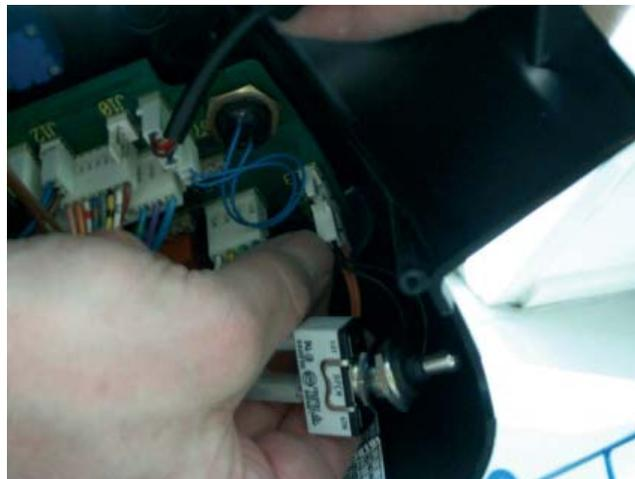
Figure 13: Connect to socket 2 on the PCB.
