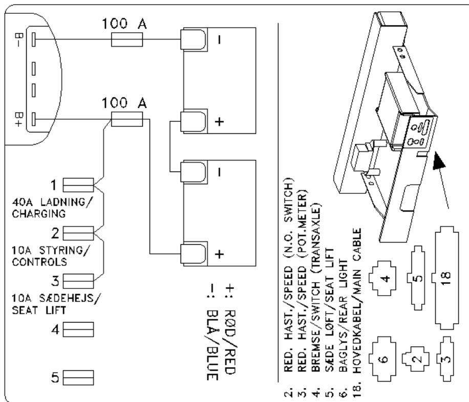
Fuses on the PCB in the operating panel. Use a pair of tweezers to replace these.
