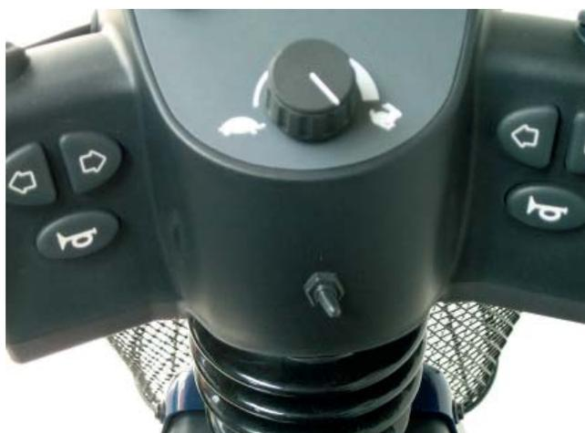
Figure 7: Install the switch so that it points to the correct side.
