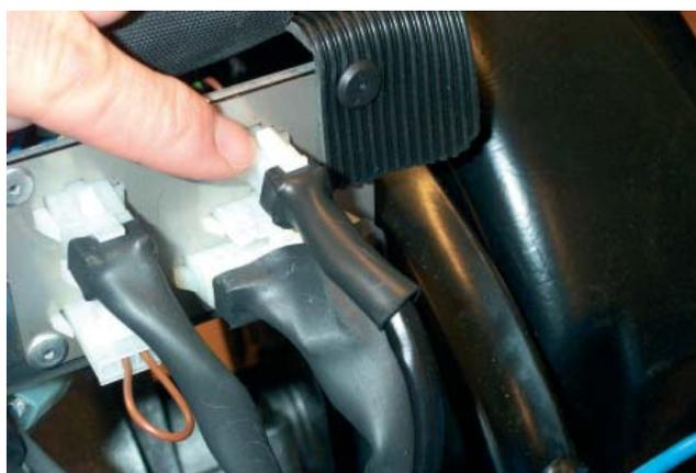
Figure 2: The four-pin plug is located above the socket area on the PCB above the motor.
