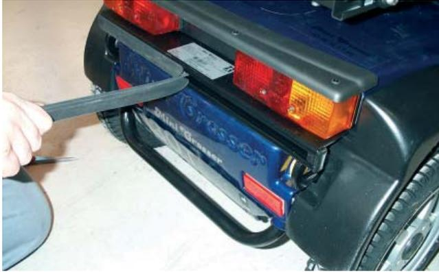
Figure 1: Remove the rubber strip in the C profile. Cut off the length that will not be used. Replace.
