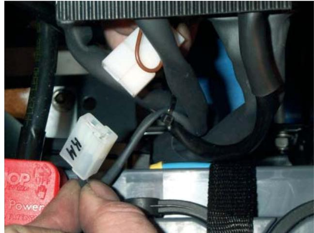
Figure 8: Connect the sensor to the socket on the aluminium plate.
