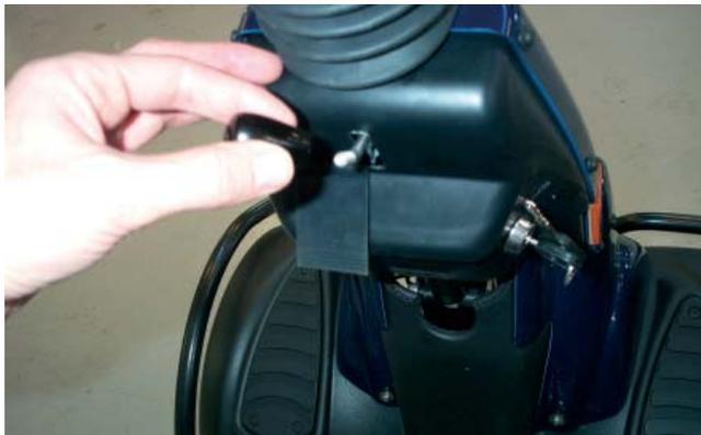
Figure 13: Remove the plastic handle.
