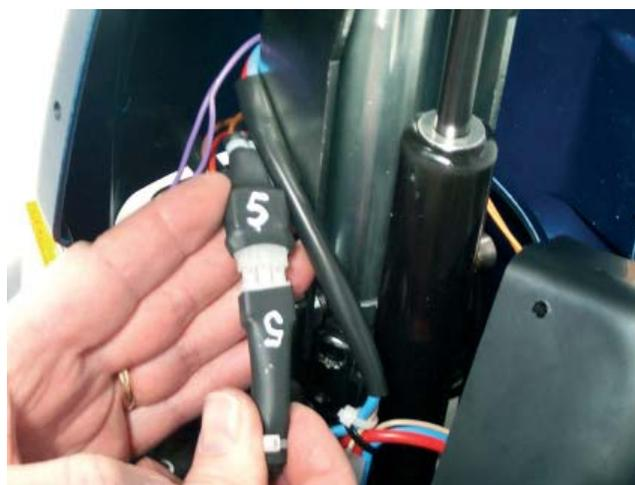
Figure 6: Connect the sensor to socket no. 5. Take care to secure the cable with cable binders so that it cannot be pinched by the front forks and/or handlebars.
