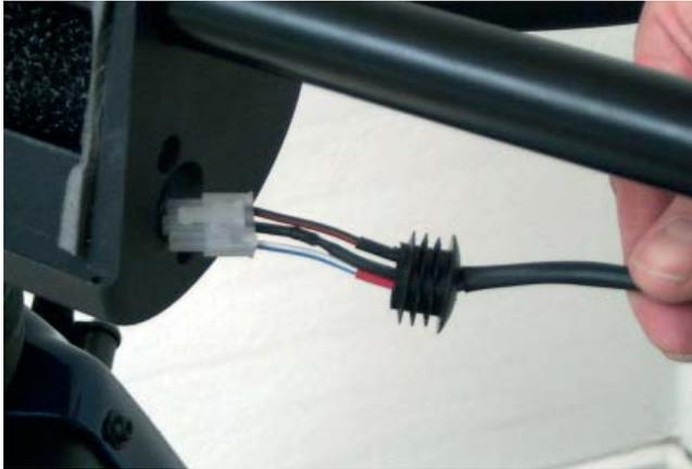
Figure 7: Install the electric plug and rubber plug in the hole.
