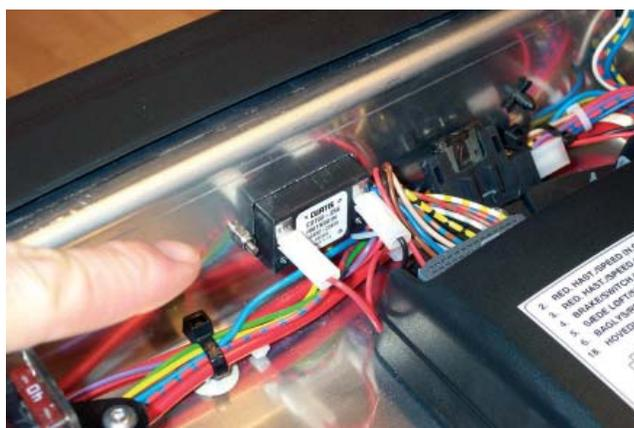
Figure 6: Install the hour counter in the pre-drilled hole in the PCB. Cut a hole in the plastic film with a retractable knife.
