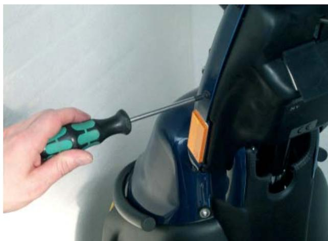
Figure 3: Remove the rear plastic shroud by removing the six plastic screws.
