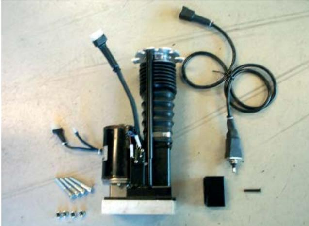
Figure 1: Complete electric seat adjustment unit.
