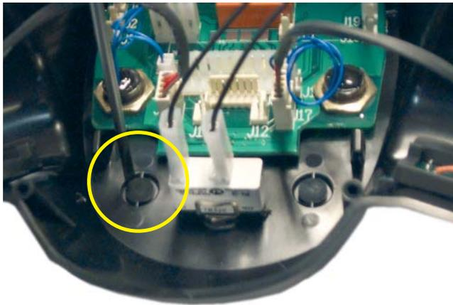
Figure 3: Cut out a hole for the reverse switch.
