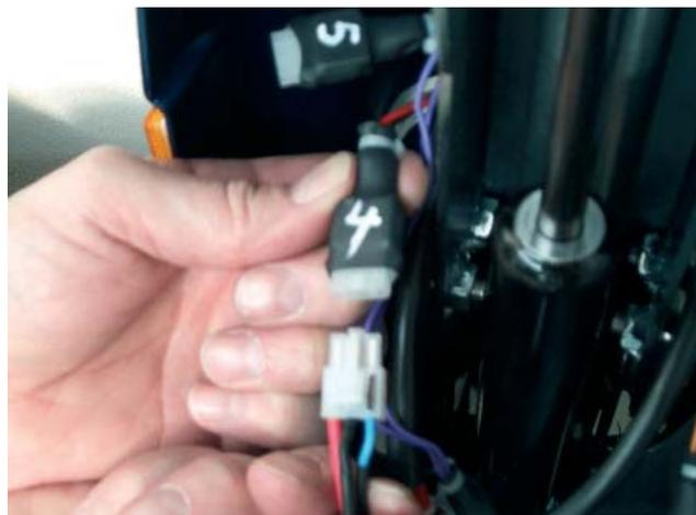
Figure 16: Connect the foot pedal throttle to socket number 4.
