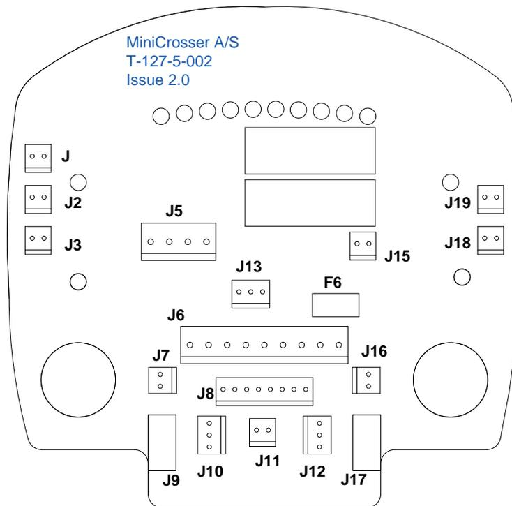
Some of the plugs on the PCB are for extra equipment. Some of them have been connected at the factory and they have been led to the areas of the scooter where they will be used. The table below shows the cases in which the operating panel should be opened. The connection for seat adjustment is not relevant to seat adjustment on the S model type. The up/down contact on the T model is also located beneath the armrest.
