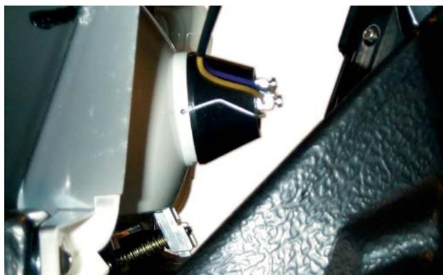
Figure 3: Lift the bracket at the back of the headlight upwards and remove it. Make sure to turn the socket in the same way again. The bracket must not touch the conductive parts of the socket.
