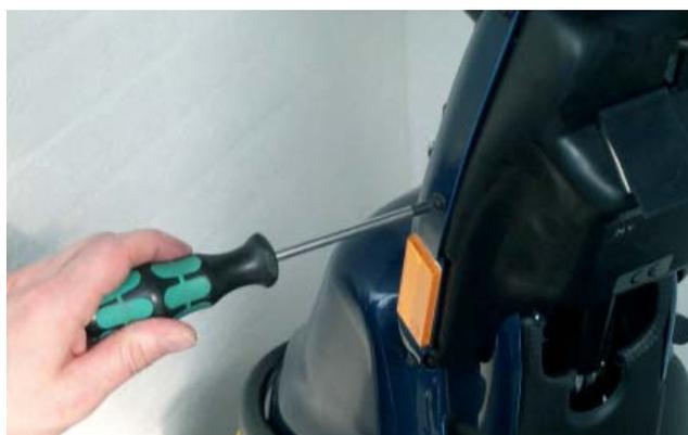
Figure 4: Remove the rear plastic shroud by removing the six plastic screws.
