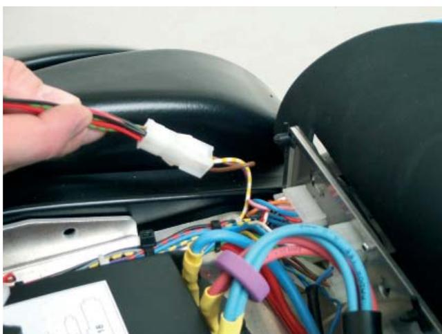
Figure 3: Remove the existing four-pin plug from the PCB. Attach one of the plugs from the hour counter.
