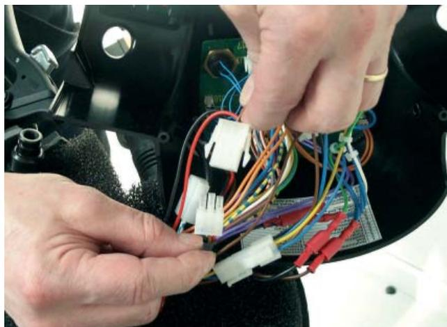
Figure 3: Remove the standard throttle regulator.
