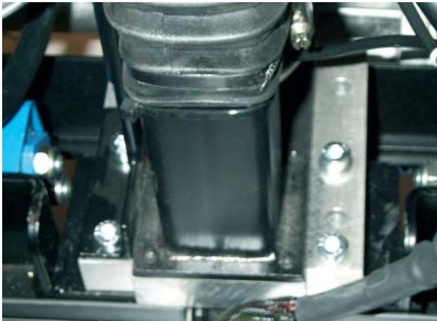
Figure 3: Install the electric seat adjustment unit in the same holes.
