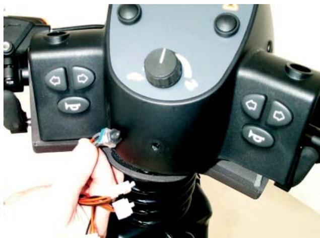
Figure 2: Remove the operating panel
