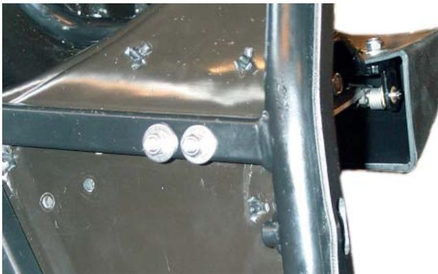
Figure 9: Install the foot pedal throttle on the footplate. Drill through the holes in the transverse square tube and up through the plastic plate and the rubber mat.
