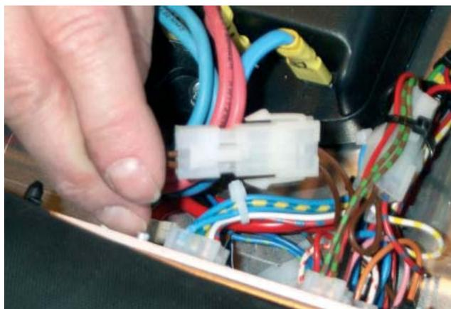
Figure 4: Install the potentiometer plug as shown. Remove the plastic cover from the operating panel as described under »Twist grip throttle – right, left». Remove the plug from the maximum speed potentiometer and install the two-pin plug with the jumper instead. Replace the plastic cover.
