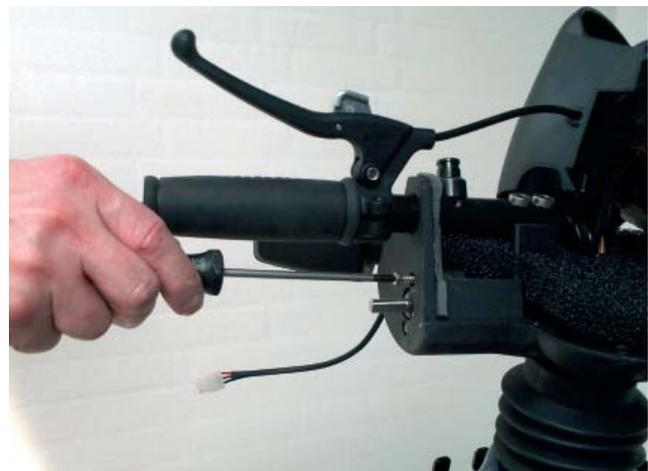
Figure 6: Remove the potentiometer.
