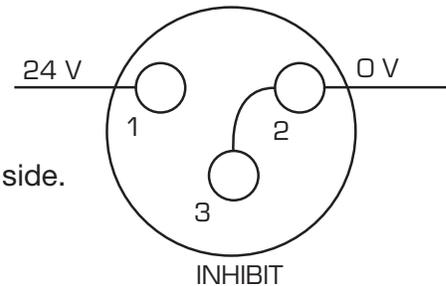
Charge plug NEUTRIK NC6MX seen from the pin side.
