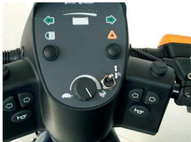
Figure 6: Install the reverse switch as shown.
