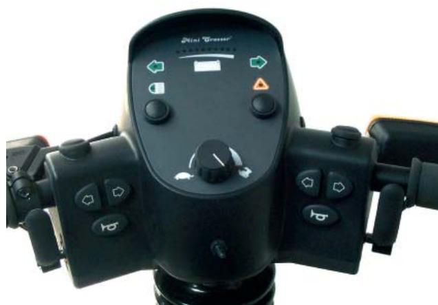
Figure 8: Install the operating panel. Take care not to pinch or stretch wires.
