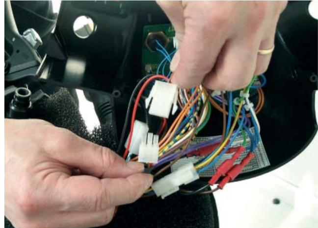
Figure 8: Connect the wires to the foot pedal throttle to the socket where the standard throttle regulation was installed.
