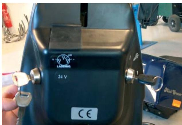
Figure 6: Replace the plastic shroud. Switch on the scooter and check that the solenoid brake clicks when the throttle is activated. When the throttle is released it should not be possible to push the scooter.
