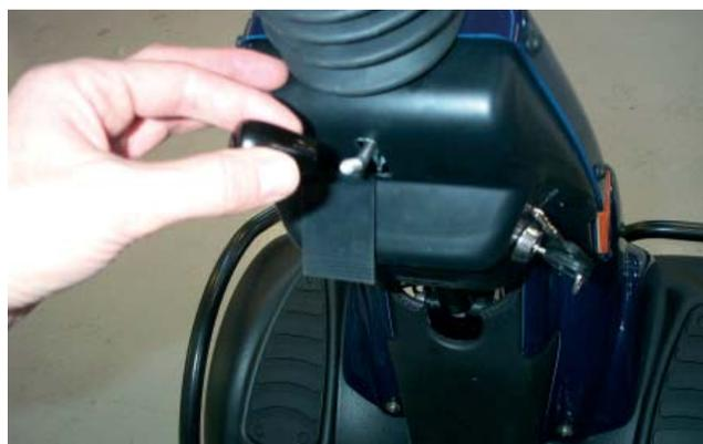
Figure 2: Remove the plastic handle from the »gas spring release«.
