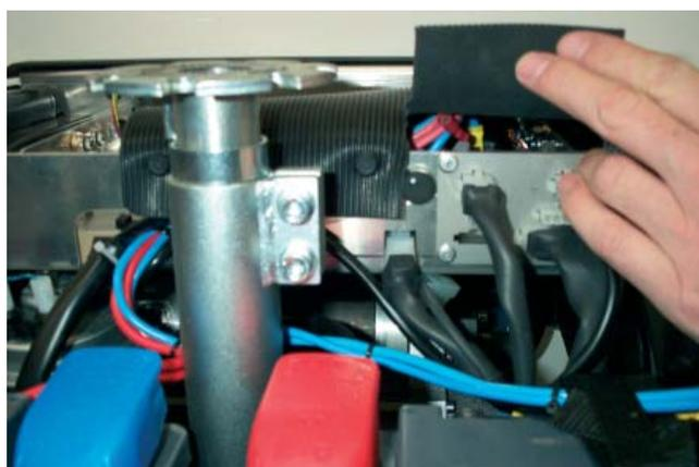
Figure 3: Install the potentiometer and push the three-pin plug out of the aluminium plate.
