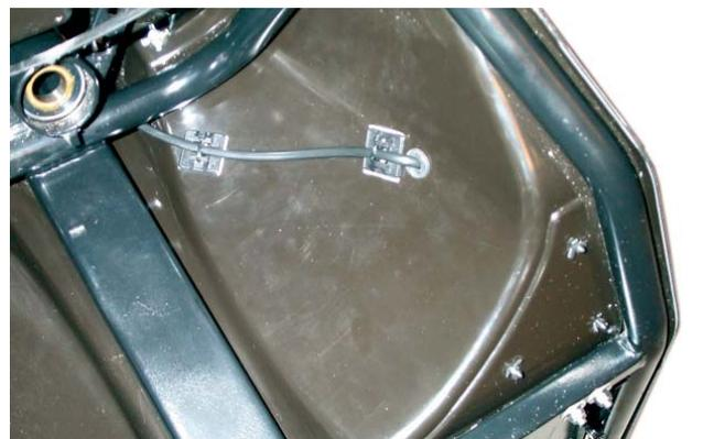
Figure 12: Install the cable beneath the vehicle.
