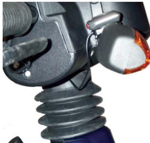
Figure 10: Connect the speedometer to the plug beneath the rubber bellows.
