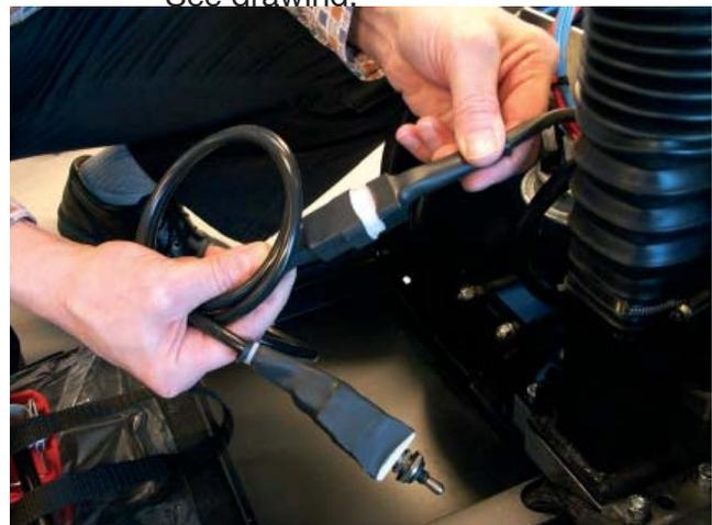
Figure 6: Connect the heavy-duty four-pin plug to the cable from the up/down switch.
