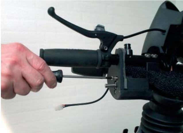
Figure 7: Remove the standard throttle regulator. Remove the rocker arm itself. If you remove the potentiometer it is important to close the holes with the accompanying plugs.
