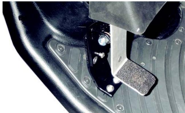
Figure 10: Connect the foot pedal throttle to socket number 4 beneath the handlebar cover.
