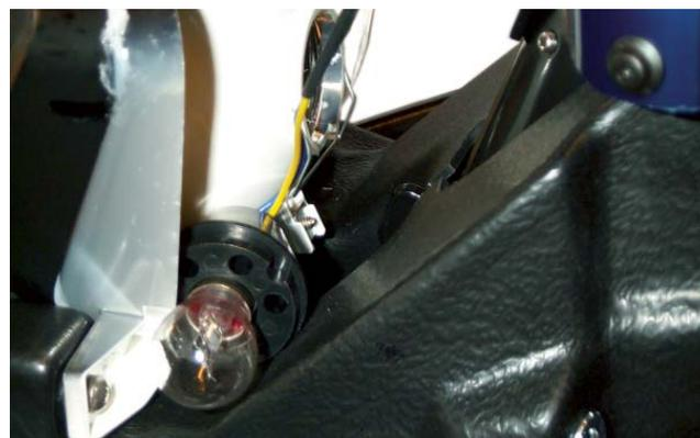
Figure 4: The socket holder can now be pulled out of the headlight assembly.
