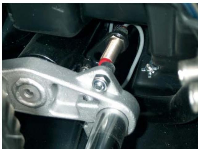
Figure 5: Adjust the height of the sensor so that it is 1 mm above the head of the bolt.
