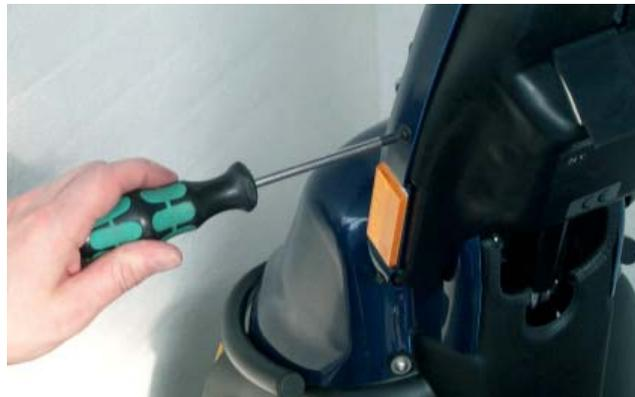
Figure 14: Remove the plastic shroud by removing the six plastic screws.
