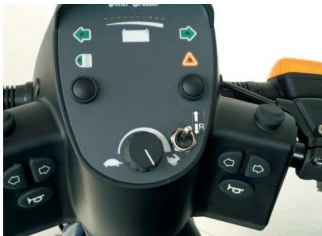
Figure 14: Install the switch and place the sticker as shown.
