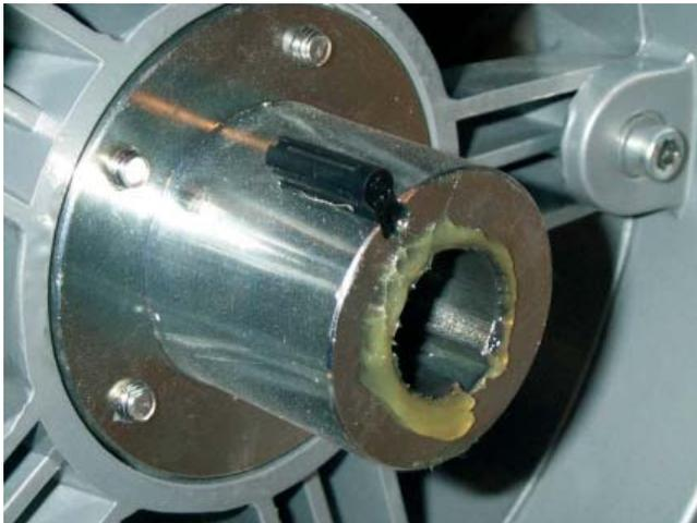
Figure 3: Install the magnet in the groove on the flange. Push in.
