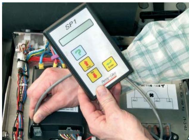
Figure 15: Program the junction box to »single-ended« input type. See separate description of programming. Switch on the scooter and check that the solenoid brake clicks when the throttle is activated.
