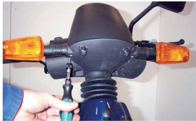
Figure 2: Open the operating panel to install the forward/reverse switch.
