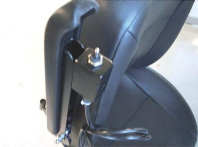
Figure 8: Install the up/down switch in the box.
