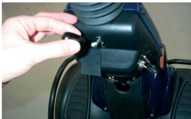
Figure 3: Remove the plastic handle.
