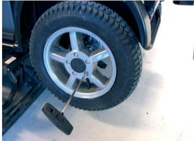
Figure 2: Remove the left rear wheel.
