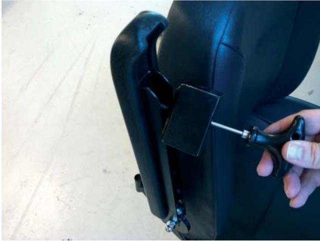
Figure 7: Install the box for the up/down switch beneath the armrest.
