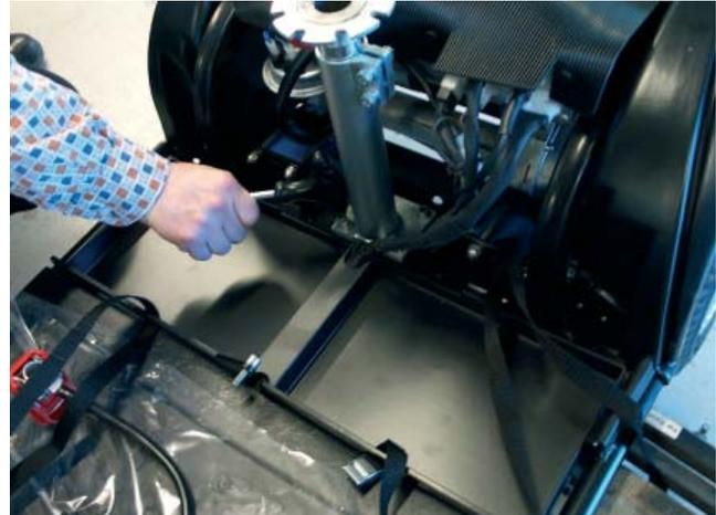
Figure 2: Remove the fixed seat post.
