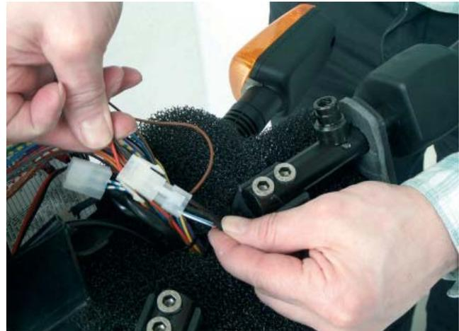
Figure 10: Connect the twist grip to the three-pin plug which the standard potentiometer was connected to.
