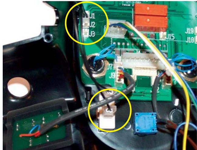
Figure 4: Connect the forward/reverse switch to socket no. 2.
