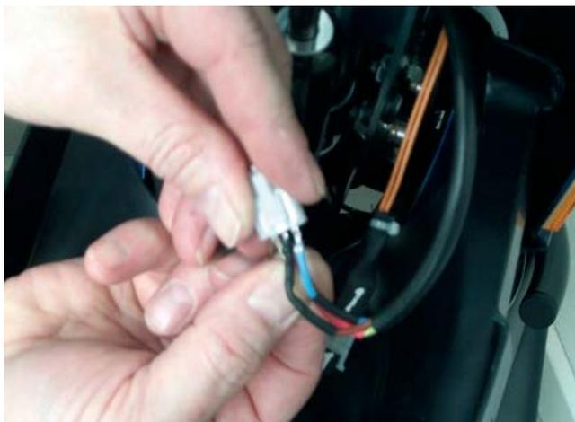
Figure 15: Insert the small crimps in the socket so that the matching colours are opposite each other.
