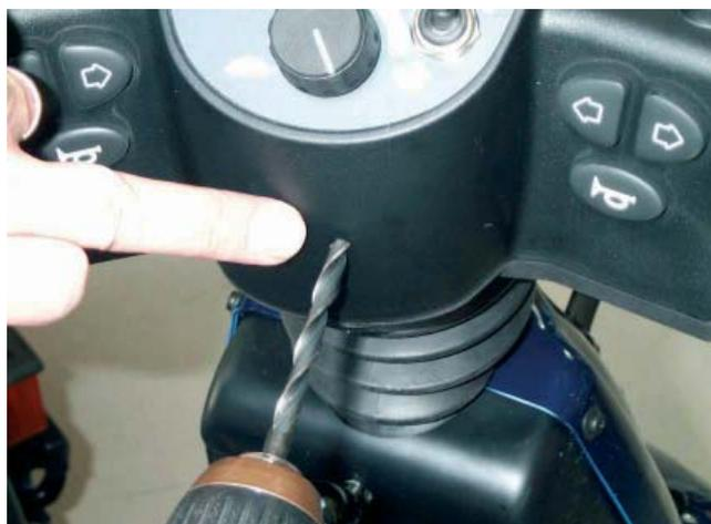
Figure 1: Drill a 6.8 mm hole as shown.
