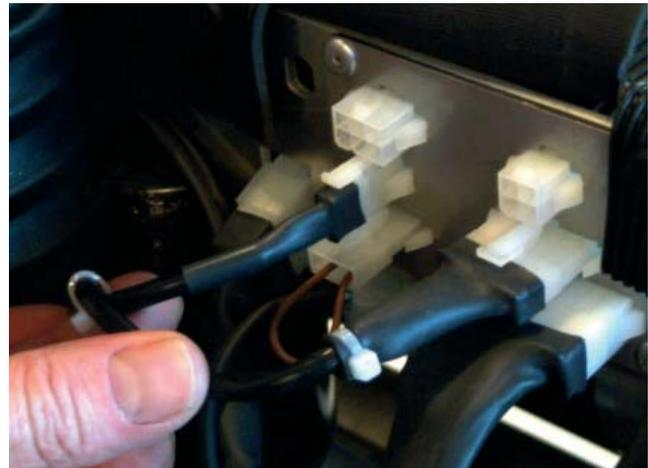
Figure 4: Connect the two-pin and five-pin plugs to the wiring plate. See drawing.
