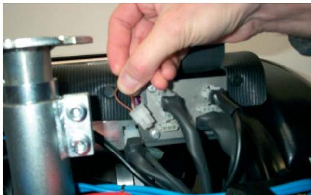
Figure 2: Remove the three-pin jumper.
