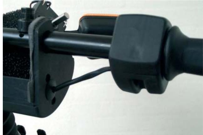
Figure 8: Install the twist grip on the handlebars.
