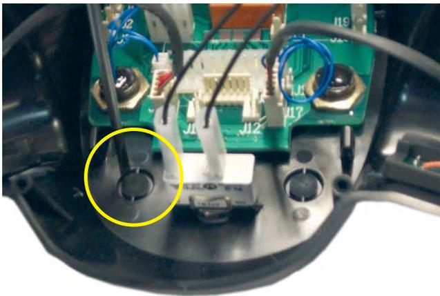
Figure 11: Install the forward/reverse switch.
