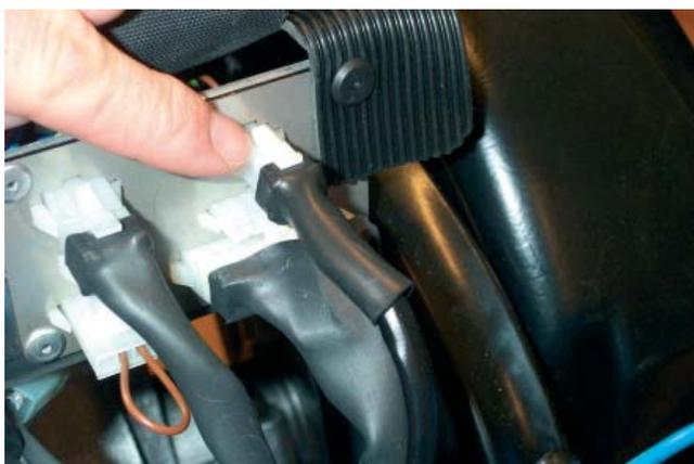
Figure 5: Replace the brake plug from the motor.
